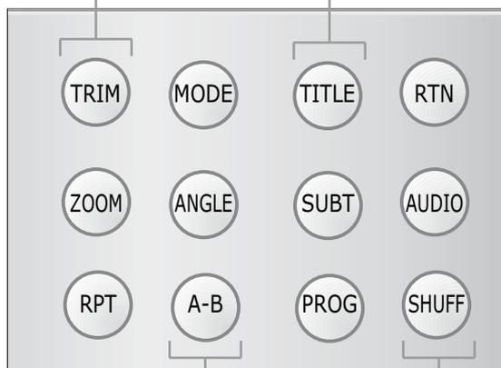
**MODE** This button brings up a menu similar to the 'Audio' page of the Set-up menu and allows the Dolby Pro Logic II settings to be changed while a disc is being played.
